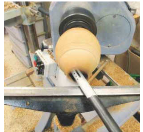
STEP 16. The tool should be worked sideways into the piece – try to establish a rhythm. Be really careful when bringing the tool in and out of the piece as you don't want to catch the fragile bark edge at this stage
